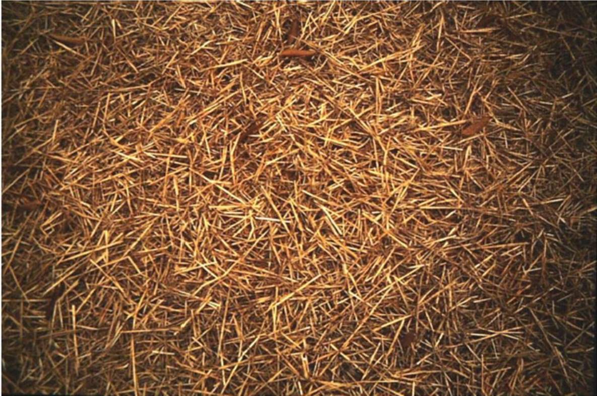
FIGURE 11.4 Straw Mulch Applied at 3 Tons/Acre
